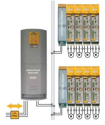
Example of a common bus system using multiple AC890 CD units with a single AC890 AFE. Bus bar connects 4 drives together with Common Bus Adapter, which connects additional rows of drives to main DC bus. The common bus adapter includes the necessary fuses.
