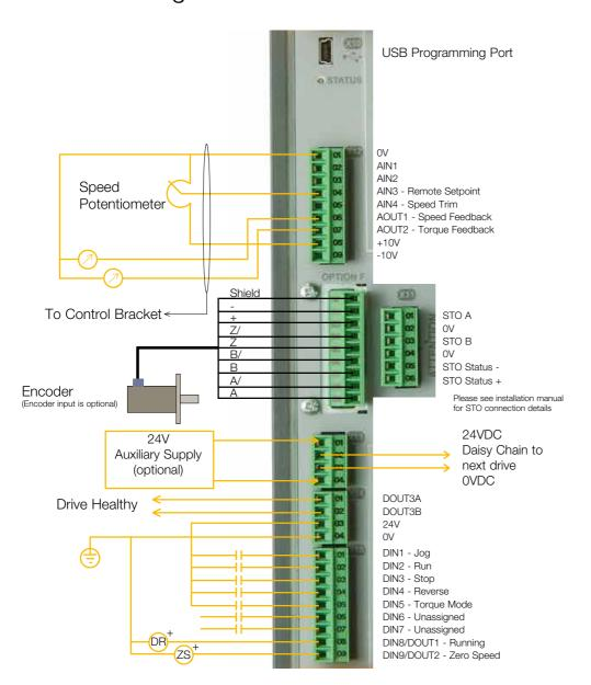
This diagram shows examples of some basic user connections to the Control Module. It is not intended to be a substitute for the installation manual which is provided with each drive and available for download on the website.
